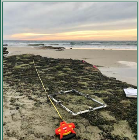
Transect (long measuring tape) and quadrat (square made of PVC pipe) set up by undergraduate students to study organisms along Narrow River.
