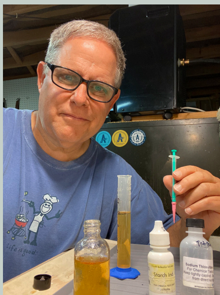
River Watch volunteer Eric Kohlsaad testing a Narrow River water sample for Dissolved Oxygen (DO). (Photo courtesy of Eric Kohlsaad)
