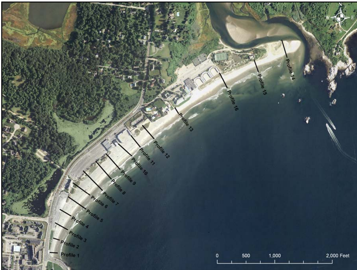
Figure 10. Beach profile and sediment sample locations surveyed on May 31, 2011.
