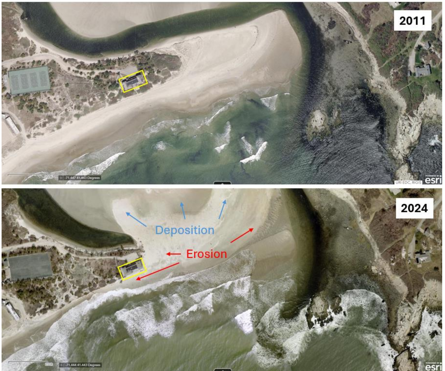
Fig. 2: Aerial images from 2011 (top) and 2024 (bottom) with text and arrows showing erosion and deposition. Erosion is also evident to the west (not shown) and has been previously documented by the RI Shoreline Change Special Area Management Plan ( https://www.beachsamp.org/coastal-erosion-maps/ ). Yellow box highlights a house that is visible in both images. Approximately 45 ft of dune erosion has occurred seaward of the house between 2011 and 2024.
