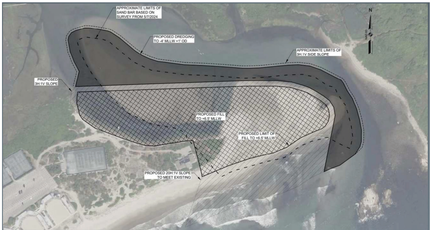
Dredge Alternative #4: Land Based dredging with Grading. Land based mechanical dredging of approximately 44,800 cubic yards (CY) of material to a depth of -4.0' MLLW + 1' of Overdepth (OD). Graphic provided by Foth Infrastructure & Environment, LLC.
