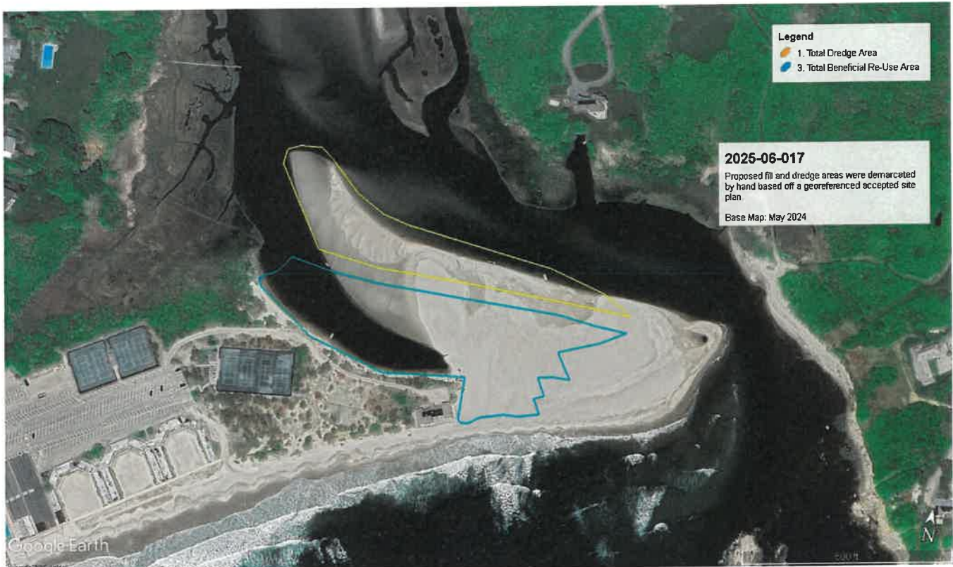
Figure 4: Dredging and renourishment areas depicted atop 2024 aerial imagery, in a similar state to present day (April 2026). Note this was after the Nor'easters of Winter 2023-2024. Dune has substantially eroded, spit has welded on to the shoal, the southern channel has closed, and the northern channel has narrowed.
