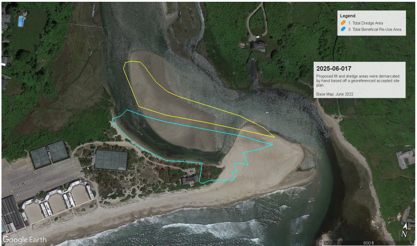
Figure 3: Dredging and renourishment areas depicted atop 2022 aerial imagery. Note this was after the Nor'easter of December 2021, but prior to the Nor'easters of Winter 2023-2024. Dune is intact and the shoal is separate from the barrier spit, but the spit has expanded north resulting in a reorientation of the southern channel and narrowing of the northern channel.
